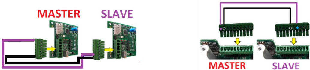
Fig. 12 – MASTER/SLAVE connection 0-10V
