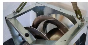
Fitting lifting lugs in the positions provided
